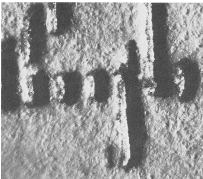
FIG. 10—The small inked vertical bar at the base of the numeral 4 on a checkwriter utilizing a ridge-and-groove format showed little embossing effect. This feature was noticed on a number of machines.
