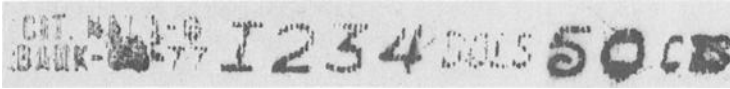
FIG. 8—The poor inking of this checkwriter caused ink diffusion and smearing. More specific idiosyncracies can also be noted, such as the variation in ink intensity in the numerals 2 and 3.
